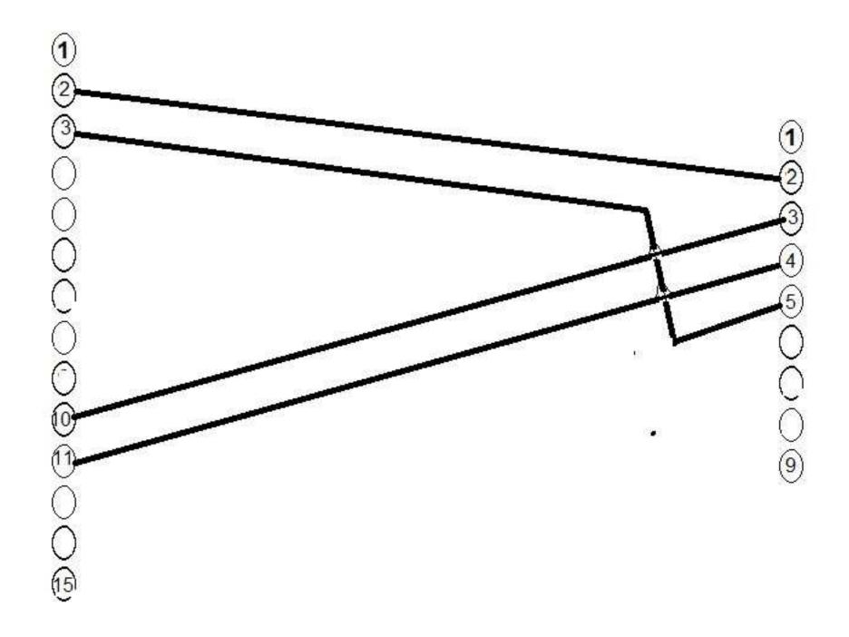
Inter Connection Between 15 Pin To 9 Pin D Shell Connector With PC To Driver
